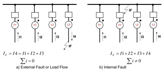
Figure 1: Bus Protection Operating Principle
